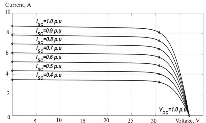
**Figure 4.** The module I-V characteristics for different short-circuit current aging factors at STC
