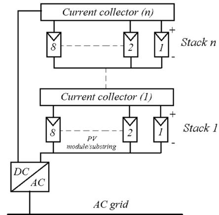
Figure 1. A schematic diagram of the CCO topology
