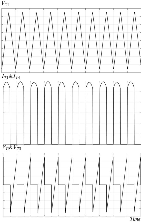
**Figure 3.** The voltage across upper condensers and the corresponding current and voltage waveforms of the SCR
