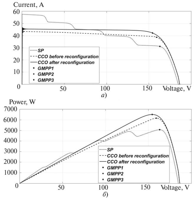
Figure 5. The characteristics of the PV array for both topologies: (a) the I-V curves and (b) the P-V curves
