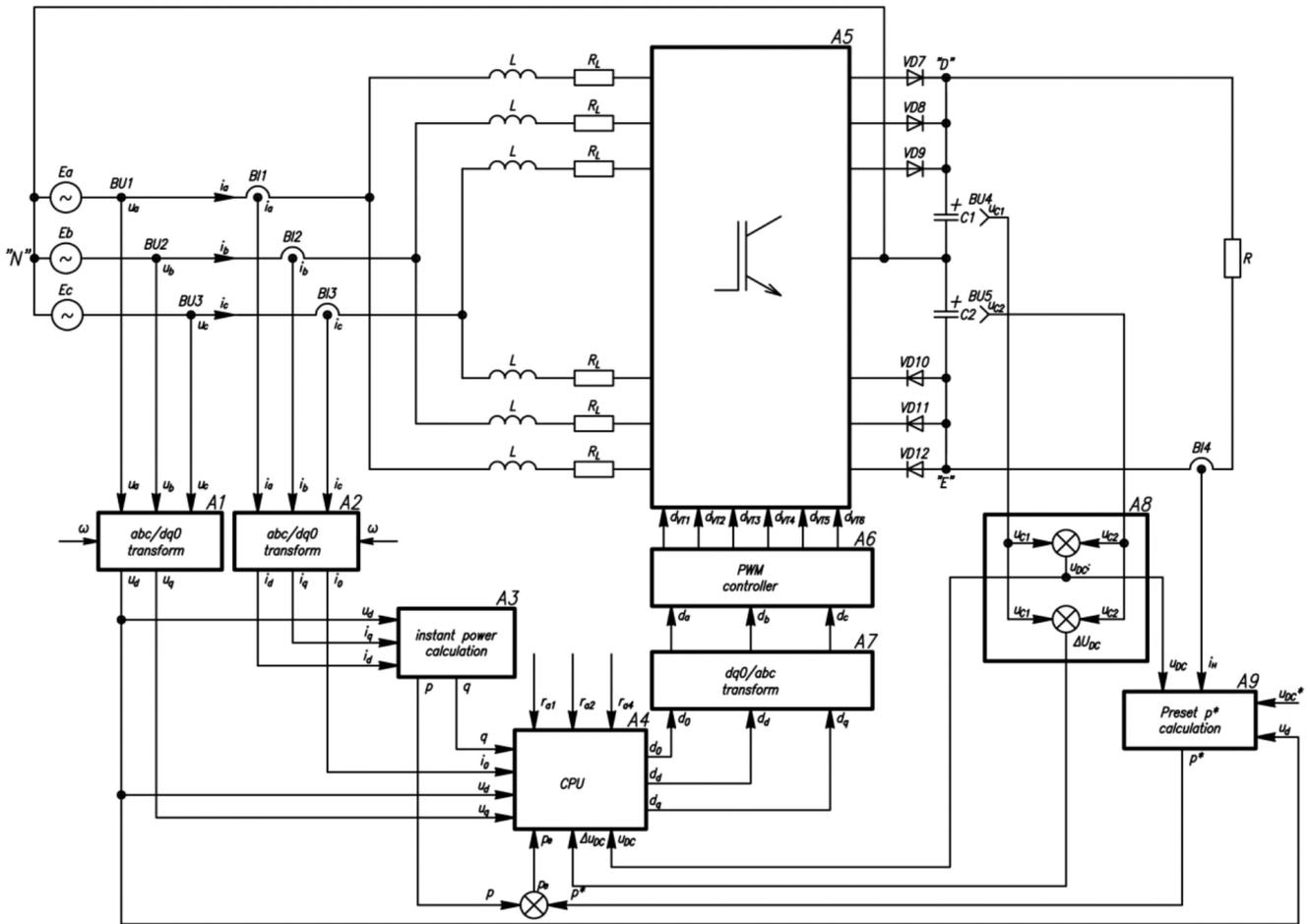
Fig. 1. The control system structure of considered three-phase PFC
